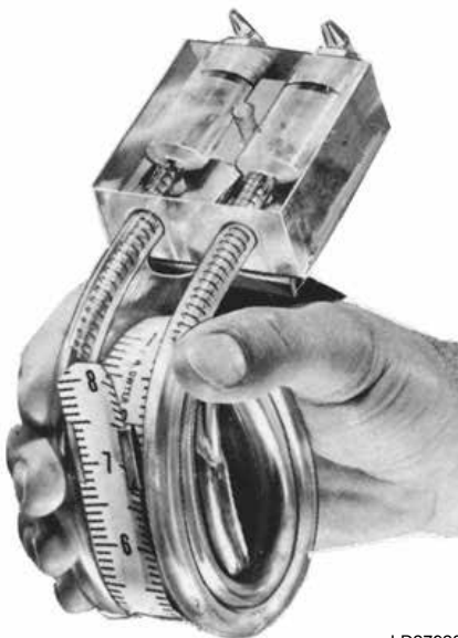
FIGURE 86 - SLACK TUBE MANOMETER
