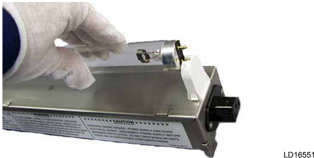
FIGURE 62 - INSTALLING V-MOD LAMP
